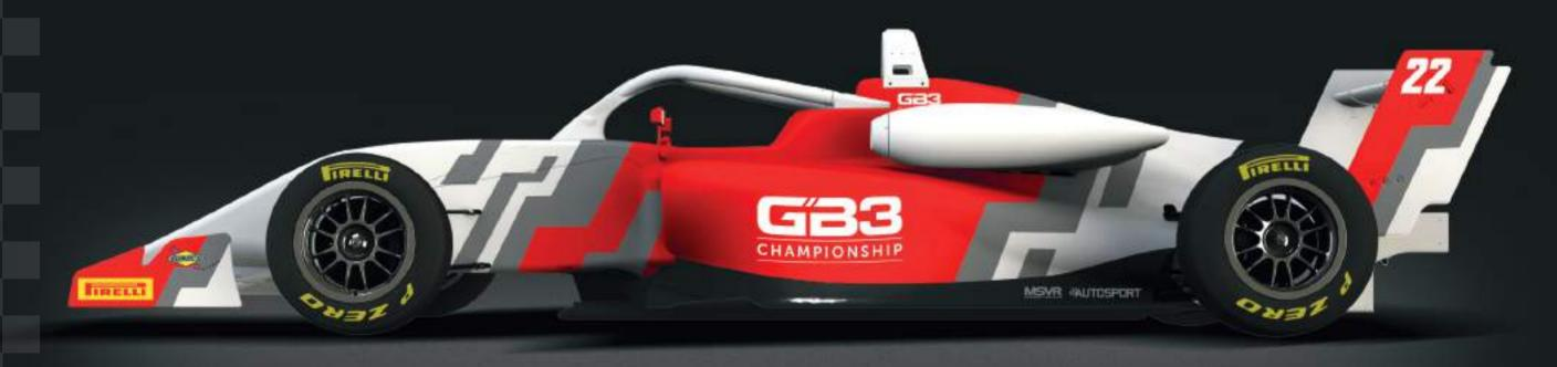
The new car of this season, the Tatuus MSV-022, will have a completely new chassis and will incorporate the halo with a new aerodynamics package completely revised.
